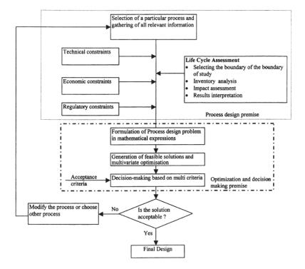
Fig.7: The basic algorithm of Green Pro (Khan et al., 2001)
